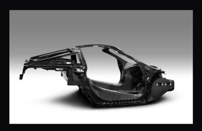
The MonoCage II features a T-shaped carbon fibre roof allowing the majority of the roof structure to be incorporated into the dihedral doors. Fitted within the chassis structure is a bespoke rollcage, designed to accommodate a repackaged interior layout with an optional passenger seat
