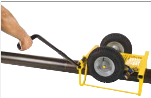
1. Use ratchet to secure Cricket to pipe
