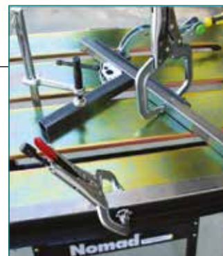
Three 28 mm slots in the tabletop allow for insertion of clamps to reach any point on the table
